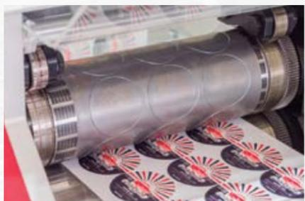
• Semi-Rotary magnetic cylinder cutting from 9 to 18 m/minute.
