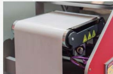
• BST Web Edge Guiding system 2 with ultrasonic edge sensor to ensure perfect aligned paper path and label rolls.
